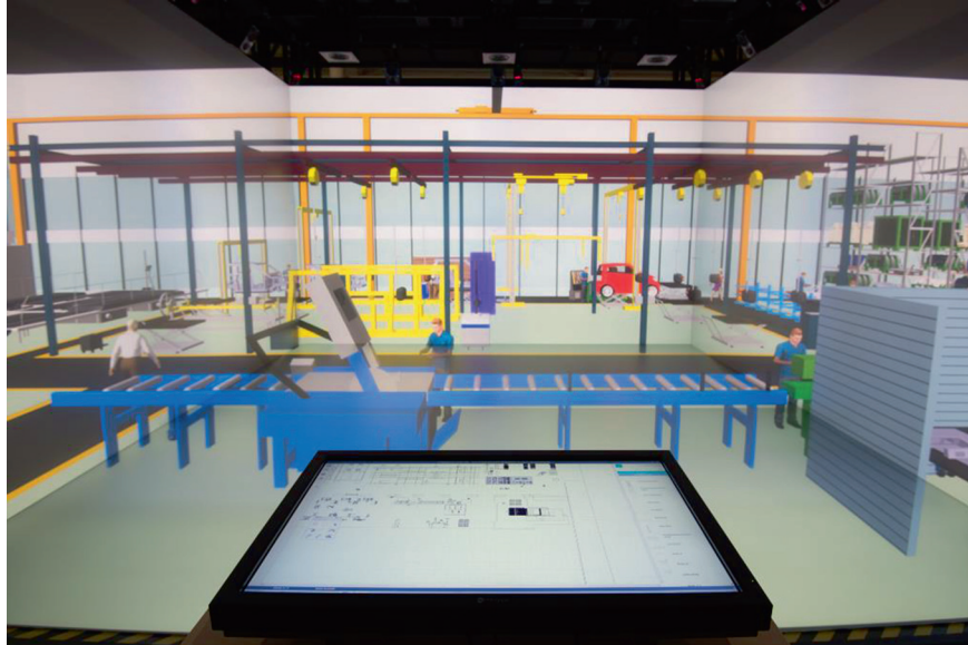
Fig. 4.12 The factory model shown in flapAssist is synchronized in real time to the one being edited using visTABLE ® touch via a network interface
