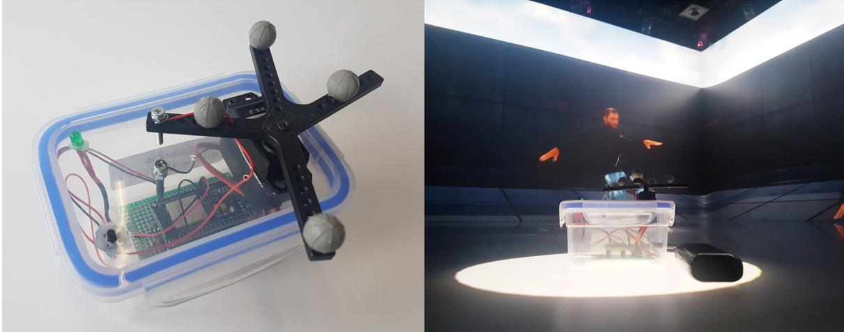
Figure 1: Left: Our implementation of the device concept. Visible are the tracking body on top, the metal contacts attached to it, the servo motor it is mounted to, the green led and the microcontroller in its bottom. Right: The device while measuring in our CAVE.
