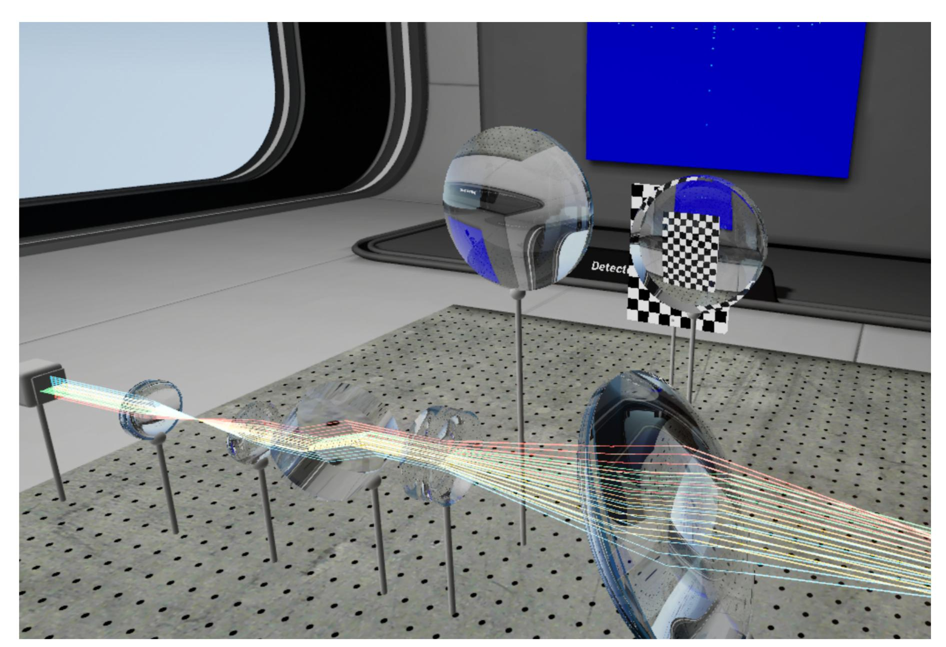
In this screenshot of the application, the optical bench with a set of spherical lenses ① is visible. The laser emitter ④ on the left emits a cross pattern through the stack of lenses, which deform the laser pattern. Additionally, the optical effect of one lens on the top right is visualized with an optical target plane ②. In the background, the resulting beam pattern is captured via the detector ③ and visualized on the wall.
