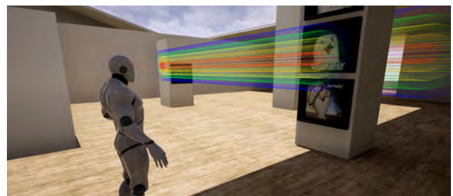
Figure 4: Detecting the user’s (represented as mannequin) interest in an exhibit by means of a conical volume of weighted rays from \omega = 0.2 (blue) to \omega = 1 (red) in steps of 0.2.
