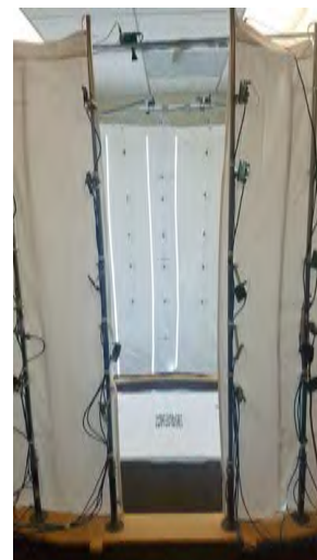
Figure 2: Photogrammetric capture cage consisting of 104 unsynchronized Raspberry Pi cameras; Designed for human body capture and used for volumetric video reconstruction.
