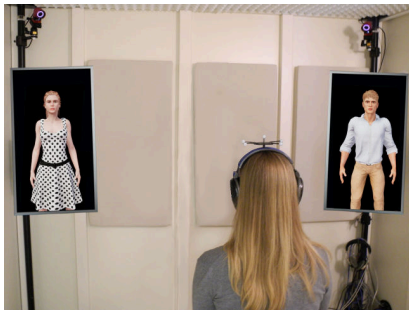
Figure 3: Experimental setup with static visual representations of the virtual interlocutors on two computer screens accompanying the acoustic stimuli of Fig. 2.
