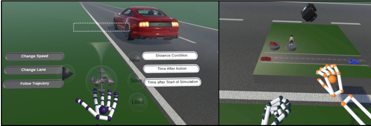
Figure 1: VRScenarioBuilder tool to author scenarios for testing automated driving features. Left: Block Editor for block-based assembly of dynamic traffic scenarios. Right: World-in-Miniature interface to navigate the scene, add and select entities (e.g. vehicle or pedestrian), and define the observer position during scenario playback.
