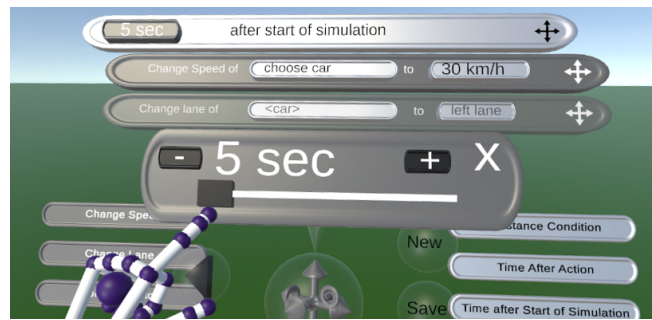
Figure 3: Depiction of VRScenarioBuilder’s Slider . The user clicked on the “5 sec” button of the Time After Start condition block. The parameter can be set by moving the slider with the index finger. The two buttons with “-” and “+” can be used for fine adjustment.
