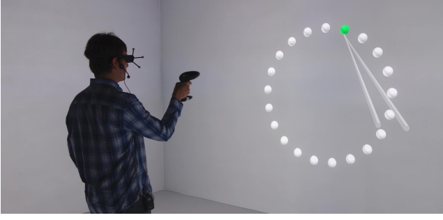
Figure 1: Experimental setup in the CAVE using a standard Fitt's law task (here T3) according to ISO 9241-400:2007.
