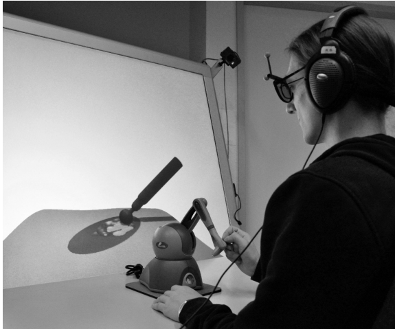
Figure 1: A participant uses a virtual drill to remove material from a surface.
