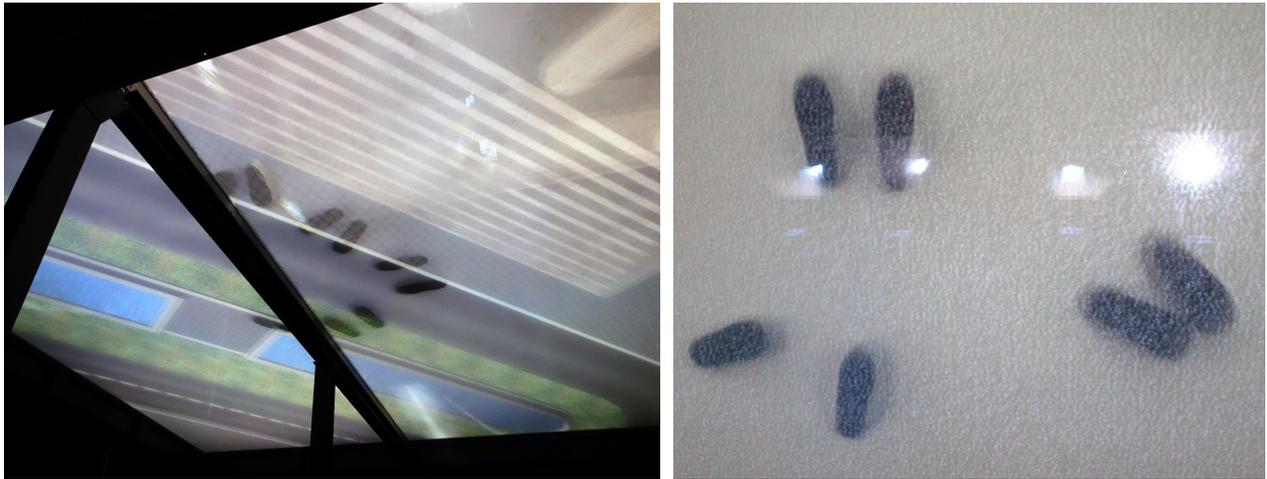
Figure 1: **Left:** Five users in a virtual scene, seen from below the under-floor projection system. The shadows of all feet are visible. **Right:** Photograph of feet in favorable conditions on the projection of a textured carpet. The white artifacts are specular reflections from the projectors.
