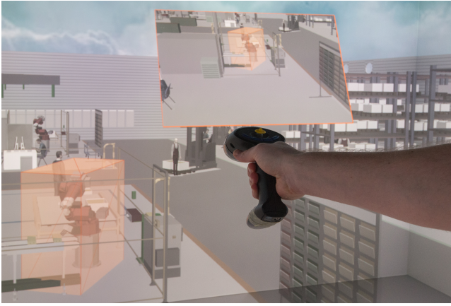
Figure 4: Interaction in flapAssist, like the SceneCamera shown here, is realized using ViSTA Widgets. Focus Strategies are extensively used to consistently combine all Widgets.
