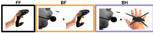
Figure 3: The 3 tested device conditions from left to right, an ART Flystick2 for clicking and pointing (FF), NVVI detection for clicking and the Fystick2 for pointing (BF), NVVI detection for clicking and an ART hand target for pointing (BH).
