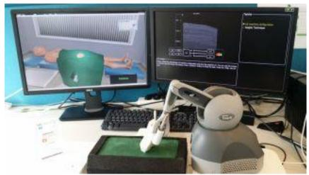
The Regional Anaesthesia Simulator (RASim) prototype shows a haptic device with the needle on a foam rest. Two screens are required for the situs (left) and the courseware (right).
